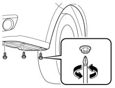
2. Turn the socket and bulb assembly counterclockwise, and carefully pull it rearward.
